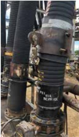
On a **built in hose nipple** - The lifting clamp should be no further than 20" behind the hose flange
